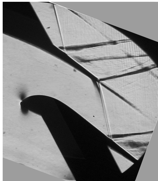
Figure 5: Schlieren picture showing shock wave/boundary layer interaction in the mid section of rotor turbine blade 48'' long at isentropic exit Mach number M_{2is} = 1.354 , incidence angle \tau = -20^\circ .
