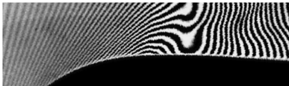
Figure 6: Detail of the Figure 4: the recompression area on the suction side, mid section of rotor turbine blade 48'', isentropic exit Mach number M_{2is} = 1.348 , incidence angle \iota = +30^\circ .
