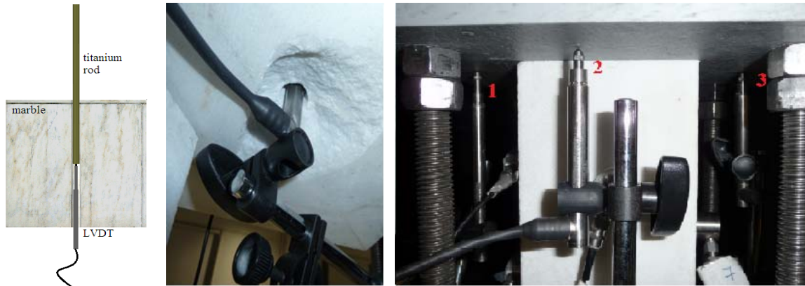
Figure 4: (a) The LVDT's position schematically (b) The lowest end of the cube (c) The LVDTs' positions under the rigid metallic plate.
