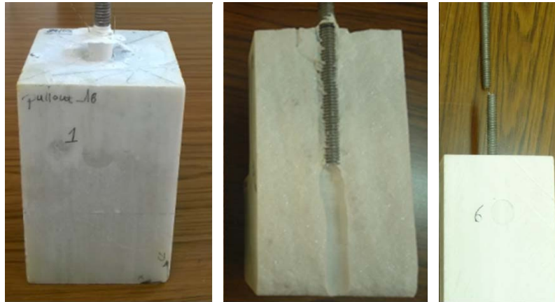
Figure 6: (a) Pullout of the bar (b) Marble's fracture (c) Bar's failure.
